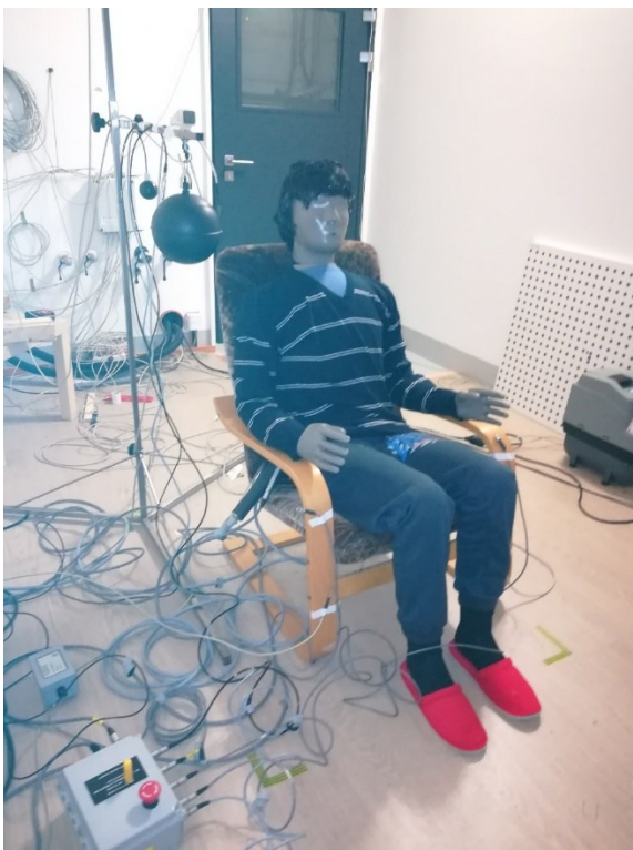
Figure 5-8 Thermal manikin with thermal comfort sensors – right side
