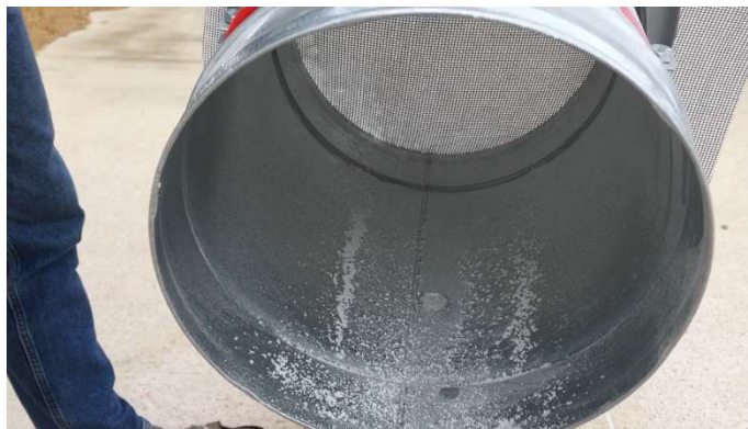
Photos of the sand cabin after fine sand particle loading
