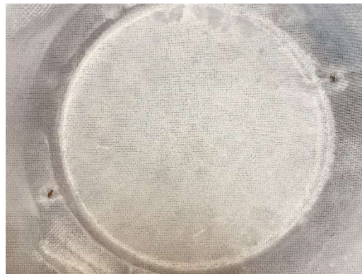
Window screen fully loaded and blocked by fine sand particle
