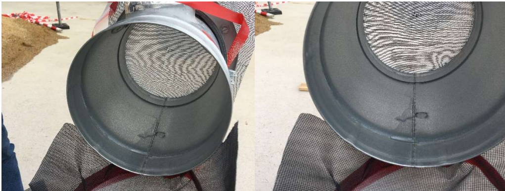
Photos of the sand cabin after medium and coarse sand particle loading
